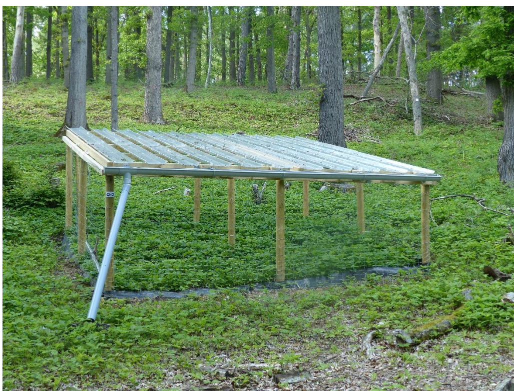
Figure 3. Partially covered roof installed above seedlings to induce artificial drought.
