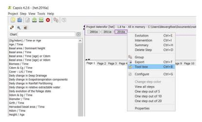
Different toolboxes are available but only three are evaluation tools: the assessment tool for the prediction of relative extractable water (REW), the assessment tool for the prediction of water content and the HETEROFOR prediction assessment tool which is dedicated to the evaluation of tree dimensional growth.
